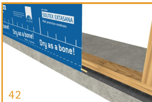
42 Leave ORCON® CLASSIC Bead with Body Thickness ORCON® CLASSIC should not be squashed flat but left with a suitable thickness to allow a flexible joint.
