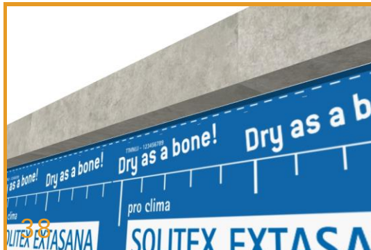
38 Staple Top Edge SOLITEX EXTASANA® SOLITEX EXTASANA® is held in place by stapling 150 mm centers leaving a 30 mm overlap onto the concrete for adhering.
